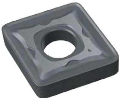
**NR2** Geometry designed for Stainless Steel Roughing. The cutting edge provides smooth cutting of Stainless Steel on high feed and high cutting depth. Interrupted cutting is also possible.
