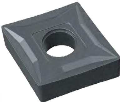
**NF32** Geometry designed for finishing and general machining of Stainless Steel. Thanks to **NF32** sharp cutting edge combined with **CM2220** grade enhanced toughness, cast iron, ligh alloy and super alloy fihishing is also possible.
